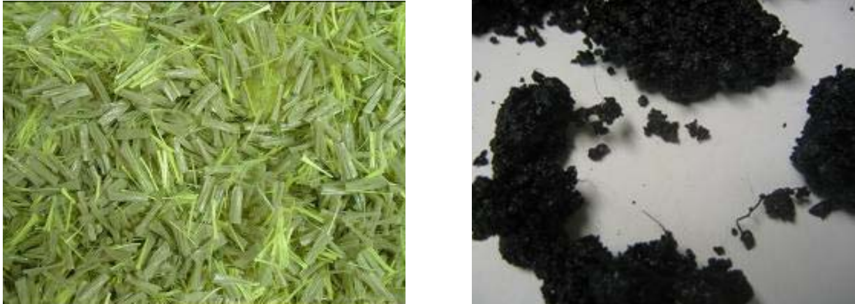
Fig. 2. (a) Close up of Reinforced Fibers: Polypropylene and Aramid (b) A Close-Up of the Fiber-Reinforced Asphalt Mixture.
