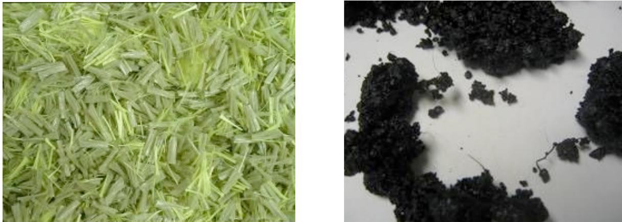
**FIGURE 2 (a) Close up of Reinforced Fibers: Polypropylene and Aramid (b) A Close-Up of the Fiber-Reinforced Asphalt Mixture.**
