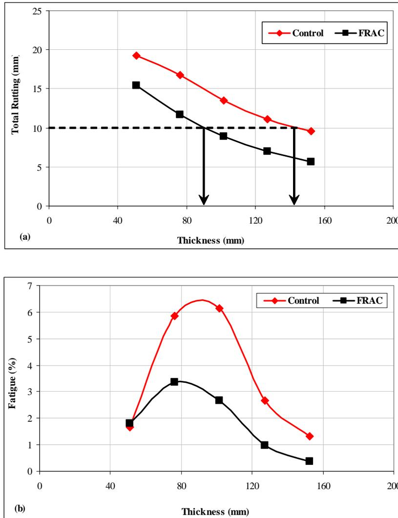
Figure 4 (a) Pavement Rutting Evaluation using the Mechanistic-Empirical Pavement Design Guide (b) Pavement Fatigue Cracking Evaluation using the Mechanistic-Empirical Pavement Design Guide.
