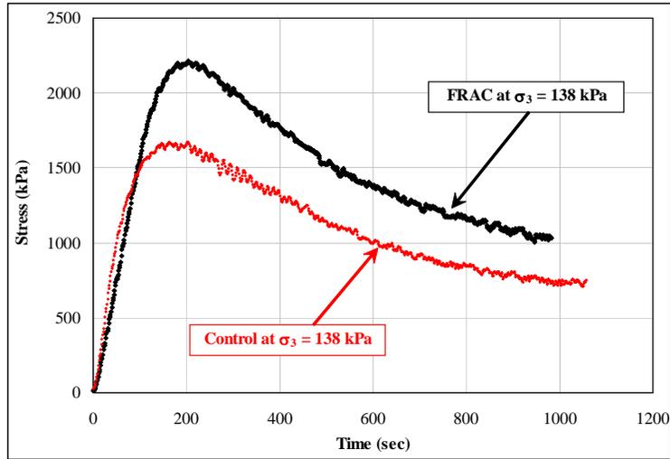
Figure 1. Comparison of Stress-Time Plots at 138 kPa (20 psi) Confinement Level.
